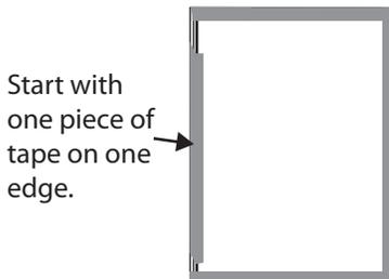
Align foam core boards together with all edges even. Use strapping or masking tape. Start with one piece on one long side to start the boards alignment -- keeping all edges even. Then continue to tape the boards together around the ALL edges.
