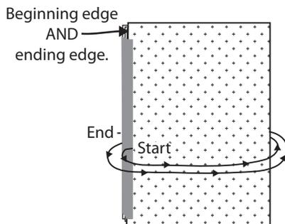
Wrap the batting around the board(s) so that the batting is exactly two layers thick on both sides and the ending edge of the batting junctions the beginning edge of the batting on the corner edge of the boards.
