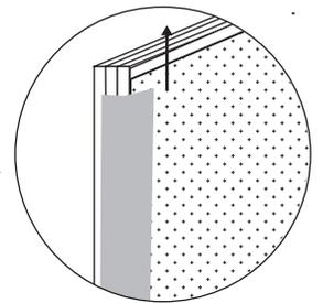
For instructional purposes, the enlargement shows the alignment of the batting along the edge of the board(s) and how to tape it in place. In actuality, the batting will extend off the top of the boards by 1/2".
